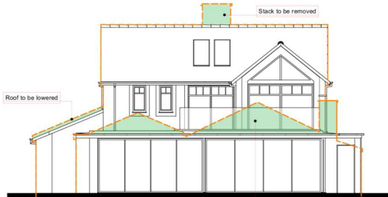
Rear Elevation_South West
